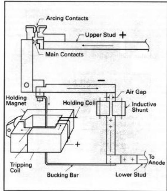
Fig. 1. Breaker Operation with Bucking Bar
